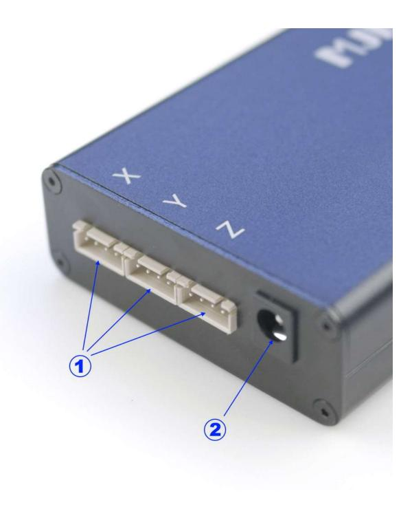
In above picture, marker 1 shows three step motor ports. Though they are labeled as X, Y, and Z, these can be changed by controlling application to something else
