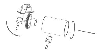
Two thin coats of paint are recommended. Be careful not to coat the threaded sections in paint. Check that the light turns and pivots as normal.
