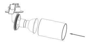
The lights are designed to be fitted to a ceiling or wall with a void. A 50mm hole saw is required. Drill the hole and connect the wiring to the house circuit.
