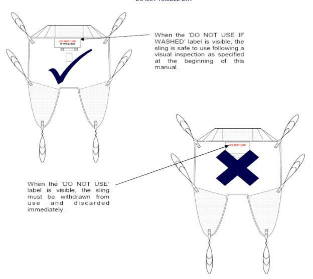
The sling can be used for bathing, but the 'DO NOT USE IF WASHED' label must remain dry. The Ink used for 'IF WASHED' is water soluble and will dissolve should it become immersed. Soiled slings should be discarded.
