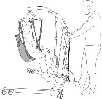
Try to position the user as low as possible (preferably resting the feet on the chassis) when transferring the lifter with a suspended user. In this way the centre of gravity will be low and reduce the risk of instability.
