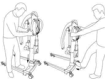
Place lifting column in chassis. Make sure that the red arrow on the lower part of the column corresponds with the edge of chassis. Make sure screw on column is inside the hole on chassis. This will prevent the column from unintentionally being lifted out of chassis when
