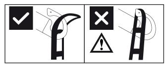
The suspensions hook design prevents sling to be inadvertently detached when mounted correct.
