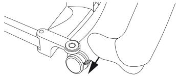
Rear wheels/castors are equipped with brakes. Step on lever to lock brakes. Flip up to unlock.
