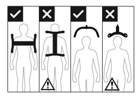
The suspension must always be positioned across the user, to prevent the user from unintentionally sliding out of the sling.
