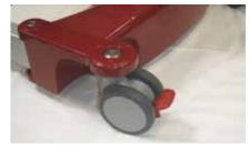
Wheels with directional lock а have no brakes fitted: we therefore recommend changing only one of the rear wheels. Push down the red lever to lock the direction. To release, pull the lever up.
