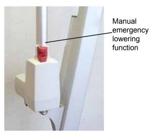
Pull the red handle up slightly. Exercise caution as the lift will move more quickly the higher the handle is pulled. Releasing the handle too quickly will increase the risk of person injury and damage to the lift.
