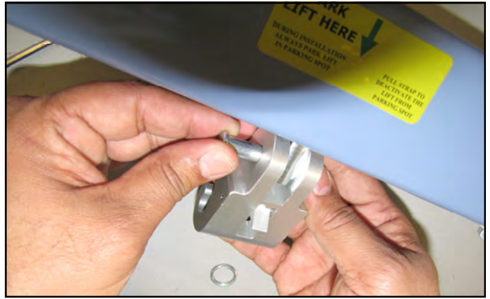
Step 2 – Detach the hook of the C-300 by taking the pin out as shown in figure .
