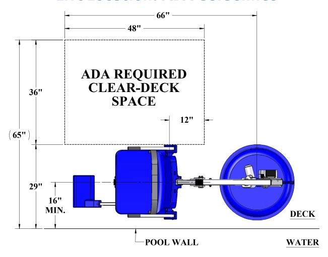
Before installing the TITAN Lift it will be necessary to select a location for the anchor. The versatility of the TITAN Lift allows it to be installed in a wide variety of locations, but the owner/installer should be aware of the requirements of the Americans with Disabilities Act (ADA) with concern to lift installations. The diagram above shows an example of an ADA compliant installation, which incorporates the following ADA rules in order to be compliant:
