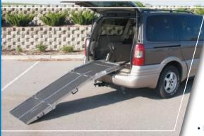
NOTE: Minimum inside door opening required for this ramp is 34". Minimum requirement for floor to ceiling opening 7' ramp - 37", 8' ramp - 41".
