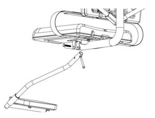
Tighten the bolt until the flat washers are snug, and then back off until the Footrest pivots freely. Adjust footrest to desired height using installed 3/8" - Button Head Bolt.
