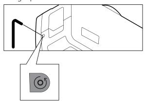
Lifter must be sent to service after performing manual emergency lowering.
