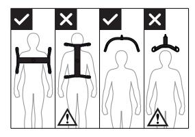
The 4-point suspension must always be positioned across the user, to prevent the user from unintentionally sliding out of the sling.
