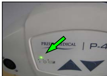
Figure 4C - When the lift has been turned "ON", the indicator light will turn green.
