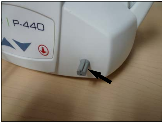
Figure 15A - Gray rubber grommet located on front right side of the lift. Rubber airline is not connected. Note ridge on grommet.
