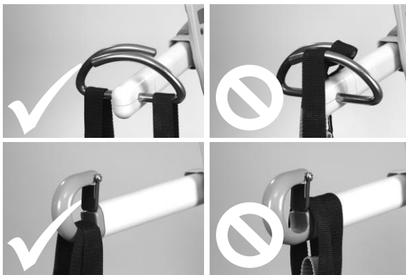
Figure 5: Sling Straps Properly and Improperly Placed
