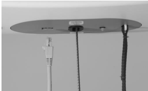
Figure 3: Hand controller connector with latch being inserted into lift connector
