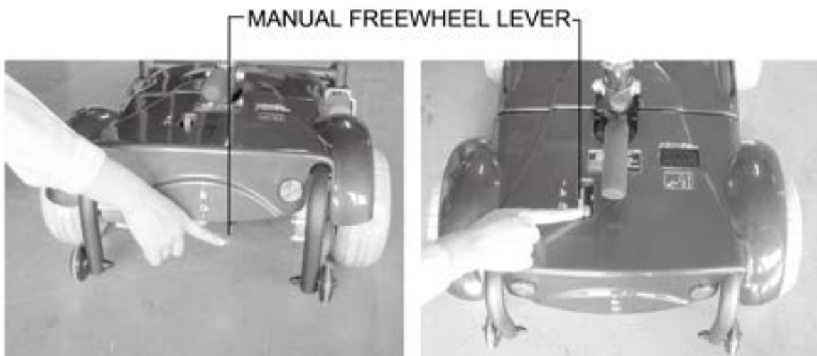
Fig J. Move release bar downward to freewheel mode. (Left motor)
