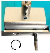
Align the 2 pre-drilled mounting hole from angle bracket with the mounting holes on the LED Panel fixture, then screw in the supplied Phillip head mounting screw by turning screw driver clock-wise.
