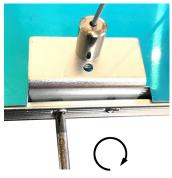
After screw in the second Phillip head mounting screw to secure angled bracket with the RGB LED Panel fixture. Repeat Step 4 for three other Angle brackets.
