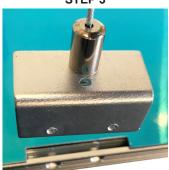
Insert the Angle bracket into the mounting slot of the back of RGB LED Panel Light fixture.
