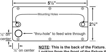
Looking from the front of the fixture the positions of through-hole and other details are reversed.
