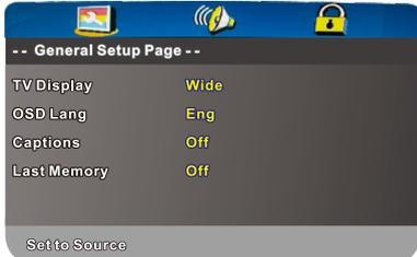
**1. TV DISPLAY:** Set the screen ratio options are: Normal/PS (4:3 Pan Scan), Normal/PS (4:3 Letter Box) and Wide (16:9). The default settings is wide.
