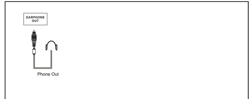
1. Plug EARPHONE out connector into EARPHONE out jack on the TV the TV speaker will be muted.
