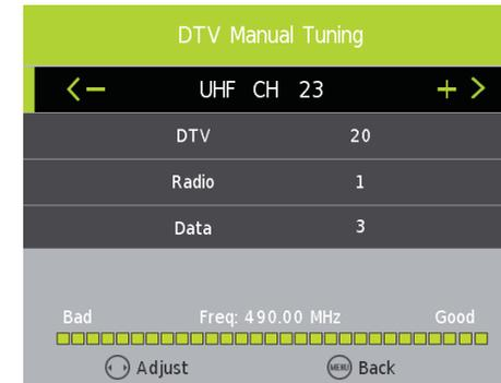
Press [LEFT]/[RIGHT] to adjust channels, when there is signal, press OK then begin DTV searching.
