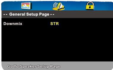
**1. LT/RT:** Logic Surround stereo audio output, This matrix-based coding process enables stereo audio tracks to carry four channels (left, center, right and surround) of audio data.
