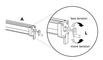
Once installed in the window, test the retraction rate.
