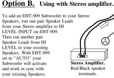
Note: there is no signal or power loss between amplifier and speakers, when "splicing-in" your EHT-909 Subwoofer.
