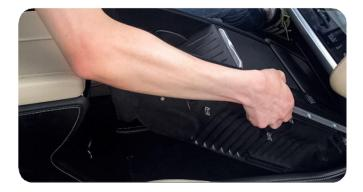
② Adjust main body to an appropriate position so power hole and USB interface can be easily used, note: for some Model S you may need to insert the center console main body as close to the car front as possible, push the rear main body down if it conflicts with the cup area (the center console rear side is soft which can be pushed)
