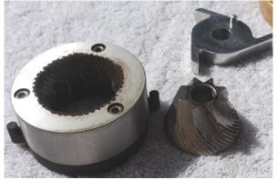
Kony has the same size burrs, in fact Kony burrs from Mazzer would just pop right in. The specially hardened food grade burrs, last 70% longer than standard hardened steel burrs. This gives less contamination as there is less wear and hence the term food grade. Burr life is in the region of 750Kg of ground coffee (source: burr manufacturer), or around 20 years home use!
