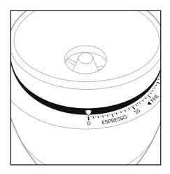
6. Rotate the bean hopper anticlockwise until the bezel ring indicator is aligned to '20'.
