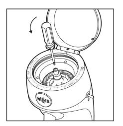
**4.** Remove the lower burr carrier from the grind chamber and place to one side.
