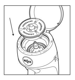
**9.** Reseat the bean hopper and screw clockwise until lightly hand tight.
