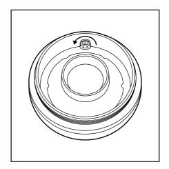
**3.** Remove the upper burr carrier and ensure that the burrs, upper burr carrier and lower burr carrier are completely clean.
