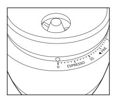
17. Once the zero point has been established, rotate the bezel ring (black ring only) until the bezel ring indicator is aligned to '0'.
