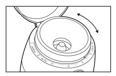
When adjusting for finer grinds, run the grinder for 1 second every time the bean hopper is rotated 10 marks on the grind dial. This ensures any trapped coffee between the burrs does not strain the mechanism and also makes adjusting easier.
