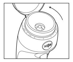
**14.** Rotate the bean hopper clockwise until the bezel ring indicator is aligned to '1'.
