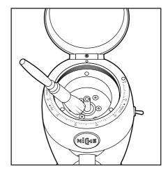
**6.** Fit the lower burr carrier from the other set and rotate until it drops to the chamber base.
