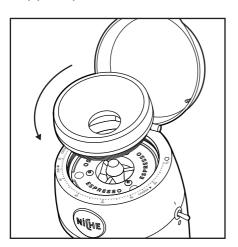
2. Loosen the thumb screw located on the inside of the bean hopper. This releases the bezel ring lock, allowing you to adjust the bezel ring.
