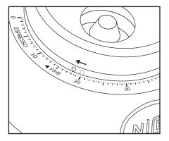
9. Close the lid and turn on the grinder for a few seconds. If the burrs sound like they are touching you are close to zeroing the burrs.
