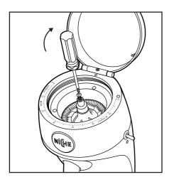
**8.** Align the three prongs on the other upper burr carrier to the holes inside the chamber.
