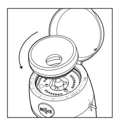
**20.** Lift the upper burr carrier out of the grind chamber and rotate it 120° until the carrier prongs are seated in the next position.
