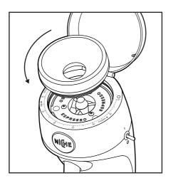
Remove the upper burr carrier from the grind chamber and place to one side.
