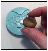
Five Star Bronze Clay is a wet clay you may use immediately after opening the package.. If the clay is drier than you would prefer, condition the clay by adding a little water and folding in thoroughly. Roll, mold and sculpt your pieces and allow to dry fully. Two pieces of clay can be connected with paste (slip). This can be achieved in the wet clay state or dry clay state. A thick paste is always better than a thin paste for attachments and regular clay is preferred whenever possible.
