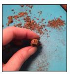
Sanding the edges and any flat surfaces should be done after the piece has fully dried. Sanding will minimize any unseen fractures on the edges thus reducing possible cracking during firing.
