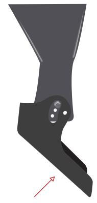
Adjust funnel at a steep enough angle that the activator can move freely up and down, and feed can slide easily down the chute.
