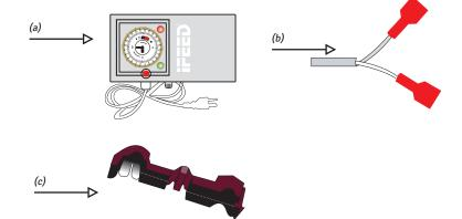
Attach the wire from the iFEED unit to the main wire using the provided purple wire clips (C).
