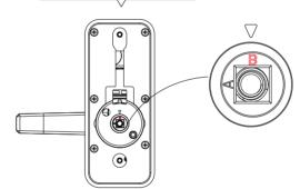
Choice of the spindle length= door thickness+18~39mm
