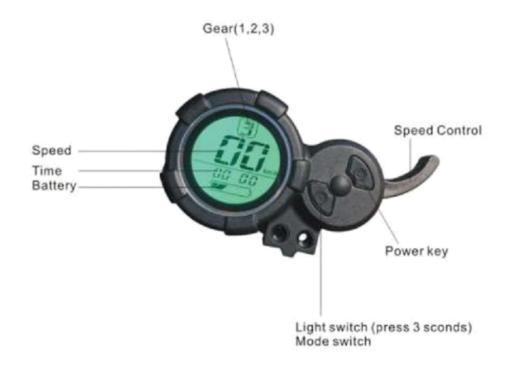
TIME: ride time for a single ride TRIP: mileage for a single ride ODO:scooter's total mileage VOL:battery voltage
