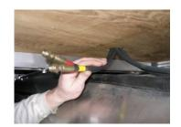
7. Run the red and black battery cables through the same hole. Route them along the backside of a cross member under the boat to an area near the transom, then up through the transom and into the battery compartment.
