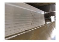
rear modules, measure from the rear most usable cross member approximately 52+forward. Mark this location with an %+:
