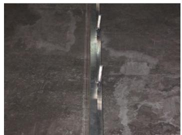
Set the left side top rail into the left upright saddle brackets. Set the right side top rail into the right upright saddle brackets. Center as desired.
