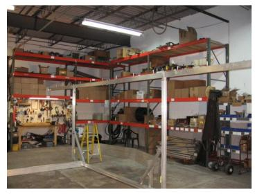
Attach the (2) top frame end rails to each end of the top rail ends using (4) 1 3/4+x 1/4 bolts and (4) 1/4-20 nylok nuts.
