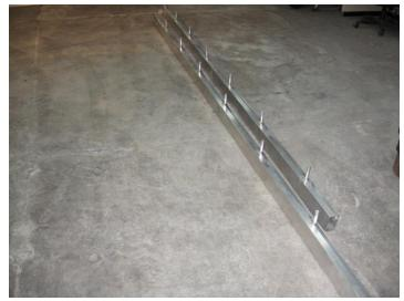
Bolt the (2) left side sections together at the splice point. Bolt the (2) right side sections together at the splice point. Each side uses (2)  $5\frac{1}{2}+x 3/8$  hex bolts, (4) flat washers, and (2) nylok nuts.
