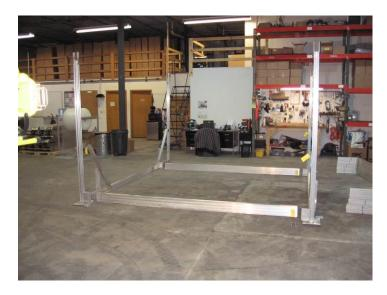
Secure the left side with (10) 3 ½+x 3/8 hex bolts, (20) flat washers, and (10) nylok nuts.
