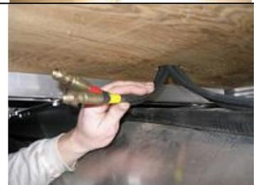
4. The hoses with blue and green bands are longer (252") and run to the front Sea-Leg. The hoses with red and yellow bands are shorter (120") and run to the rear Sea-Leg.
