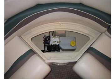
2. Place the pump in your chosen compartment, and select a spot near it through which to drill a hole to feed the Sea-Legs hydraulic hoses under the boat. Remove the pump and drill a 1/8" pilot hole to insure clearance above and below deck – *be extremely careful not to puncture the pontoons nor hit any wiring.* If the pilot hole proves satisfactory, drill a 2" hole through which to feed the hoses.
