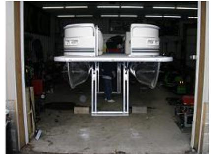
18. Press BOAT DOWN on the remote to lower the boat. Always keep an eye on the oil level in the reservoir tank, and continue to add oil if it drops below half full. At this point you only want a half full tank as the oil is flowing back into the reservoir tank.
