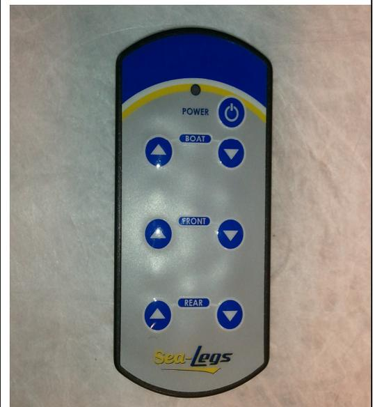
NOTE: You may find that the front of the boat rises faster than the rear. This is normal and to be expected, as the majority of the boat's weight (particularly if fully rigged) is in the rear of the boat. In order to keep the boat level during ascent and descent, you may need to toggle between FRONT UP and REAR UP buttons on the remote.
