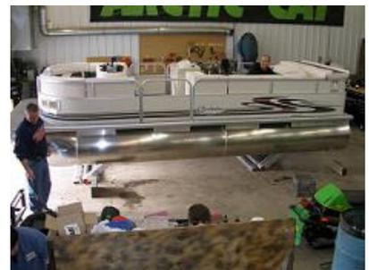
off the shop floor (or ground). Continue raising the boat until it begins to lift off of the rear blocks. **STOP**. Check all rear hoses/fittings under the boat for leaks.
