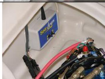
6. Secure the remote control receiver to a **vertical** surface using the four (4) #8 x 3/4" screws provided. Avoid placing the receiver near speakers as it could interfere with the remote control operation.
