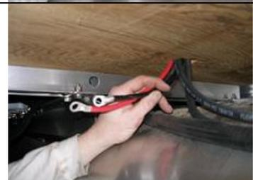
5. Run the red and black battery cables through the same hole. Route them along the backside of a cross member under the boat to an area near the transom, then up through the transom and into the battery compartment. (If the battery compartment is adjacent to the Sea-Legs pump compartment, you can run the battery cables through a hole between the compartments.)
