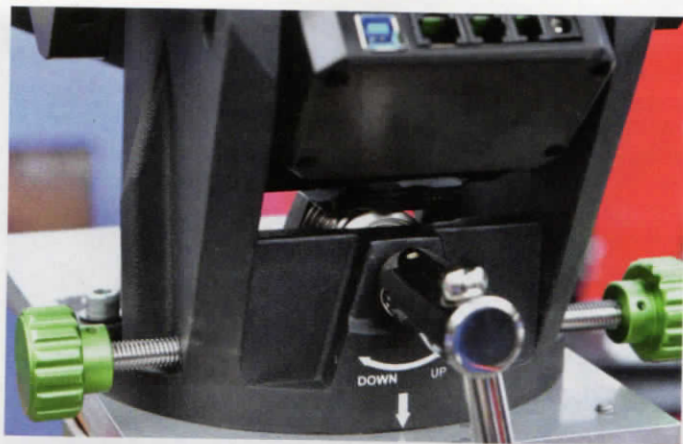
▲ Left: The mount's polar alignment can be precisely adjusted with heavy-duty controls on the azimuth and altitude motions of the polar axis. Right: While the EQ8-R Pro has an optional polar-alignment scope available, the author used its mounting cap screws to attach his QHYCCD PoleMaster to electronically dial in the mount's alignment.
