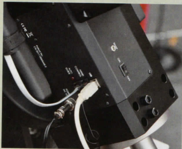
◀ Described in the accompanying text, the EQ8-R Pro has an internal cable-management system for power, USB 3.0, and modular-jack cables. Input ports (far left) on the fixed end of the polar-axis housing have corresponding outputs on the declination saddle (middle, only one end shown). The mount's power, autoguider, and computer USB connections (left) are on the side of the declination-axis housing.
