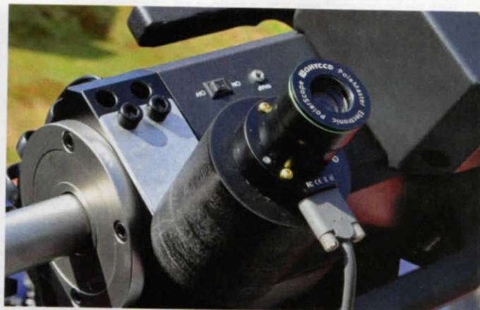
▲ Left: The mount's polar alignment can be precisely adjusted with heavy-duty controls on the azimuth and altitude motions of the polar axis. Right: While the EQ8-R Pro has an optional polar-alignment scope available, the author used its mounting cap screws to attach his QHYCCD PoleMaster to electronically dial in the mount's alignment.
