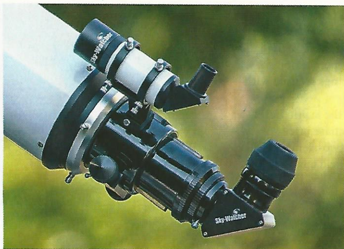
▲ Left: The telescope's solid 3.4-inch rack-and-pinion focuser and mounted 8x50 right-angle finderscope are rotatable by loosening the large metallic "captain's wheel" ring with machined spokes. Right: A millimeter scale to aid in repeating focus positions is printed on the focuser drawtube. Also visible is the 10:1 fine-focus knob.
