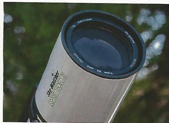
▲ The telescope's 150-mm f/7 (1,050-mm focal length) air-spaced, three-element objective incorporates one element made with FPL-53 extra-low-dispersion glass and two BK7 elements. Its retractable dewshield is secured with two thumbscrews.
