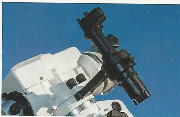
An outboard polar alignment scope bolts securely to the mount, replacing a small bubble level used in alt-azimuth mode. The separate “bright field” illuminator is shown on the front of the polar scope.
