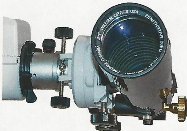
The secondary saddle has two fine adjustment knobs for aligning the second telescope in altitude to match the field of the main telescope. No adjustment capability is provided for azimuth, though none was needed.
