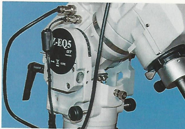
The AZ-EQ5 comes with excellent azimuth and latitude adjustments for precise polar alignment. The latitude adjustment range spans from 0° to 90°. The ribbed black wheel (seen on the counterweight shaft) is the declination lock. Note the secure locking plugs for the declination and power cables, a professional touch.
