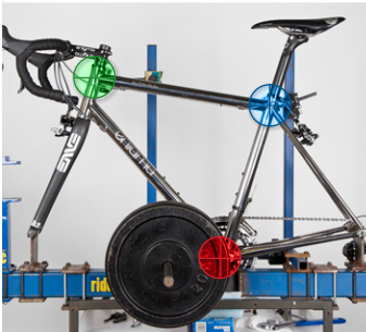
Hexagonal half cap? That's what we'll call this tidy drop-out design. Light and strong with plenty of surface area for welds. Pairing this frame with a quietly excellent parts kit results in an excellent all-round machine, or what we used to call a road bike.
