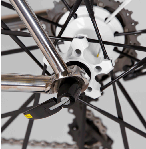
Hexagonal half cap? That's what we'll call this tidy drop-out design. Light and strong with plenty of surface area for welds. Pairing this frame with a quietly excellent parts kit results in an excellent all-round machine, or what we used to call a road bike.
