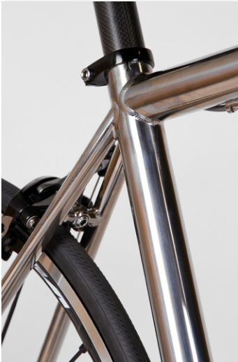
It might not win a side by side comparison against a certain titanium master from Geelong, but the weld quality on display in the Enigma is certainly of a very high standard.
