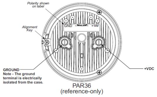
Figure 10.1 – Typical PAR36 LED Light
