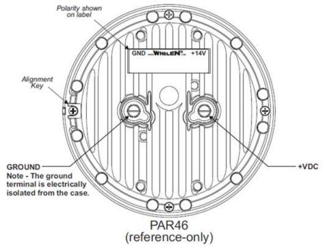
Figure 10.2 – Typical PAR46 LED Light
