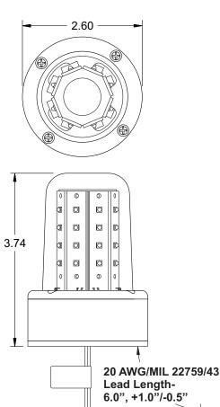
SJS840351 Connector POS A = 28VDC, WHT POS B = Ground, BLK POS C = N/C
