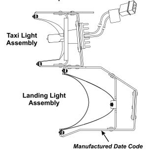
Step 2 - Locate, remove and retain the four (4) nuts, flat washers and socket head bolts that secure the taxi reflector to the assembly. Remove the taxi reflector from the assembly.
