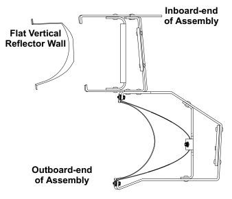
Step 4 - Position the new reflector onto the assembly and secure with the original hardware. Wipe the mirrored surface of the installed reflector with a clean soft lint-free cloth to remove any fingerprints or contaminants. Re-install the light removed in step 1. Re-install completed assembly
