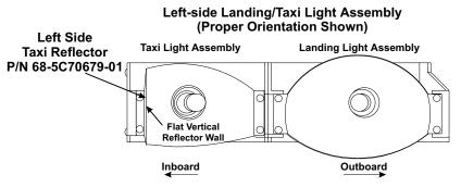
When inspection of the left Landing/Taxi light assembly is completed, proceed to the right Landing/Taxi light assembly. As shown, the flat vertical reflector wall should be oriented so that it is in the inboard position.
