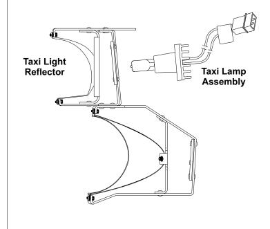
Step 3 - Obtain the correct reflector for the taxi light. When properly oriented, the flat vertical reflector wall will be positioned at the inboard end of the assembly and the lamp opening will be aligned with the lamp mounting opening in the assembly.
