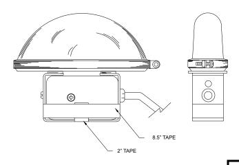
ATTACH 2" LONG PIECE OF TAPE AS SHOWN, ALIGNED WITH PART CENTER.
