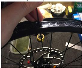
7. Remove dust cap and push valve through the valve hole
