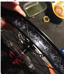
6. Use a small spike to pierce the tape in the centre of the valve hole
