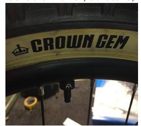
11. Deflate the tyre fully, taking care to keep the tyre bead fully seated on the rim, shake the packaging vigorously before every use to ensure an even distribution of platelets
