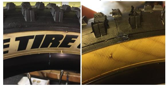
15. Give the wheel a good shake to disperse the sealant around the wheel or better still, GO RIDE! This will disperse the sealant around the inside of your tyre and rim sealing any small gaps.
