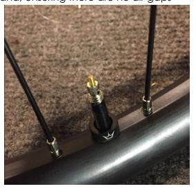
9. Slot the valve cap over the valve core, Twist anticlockwise until the core can be pulled out
