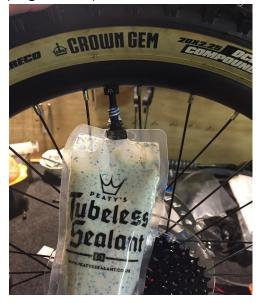
13. Re-insert the valve core and re-inflate the tyre to desired pressure.
