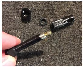
8. Install O-ring - Apply lock ring tightly by hand, ensuring there are no air gaps
