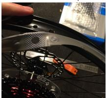
5. Starting at least 10cm before the valve hole, Press the tape firmly into the centre of the rim and smooth out to the edges, removing any trapped air. Run tape around the rim while keeping tape tension and allowing for at least 10cm overlap of tape at the end when cut
