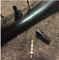
10. Seat both sides of your tyre onto the rim and inflate initially with no sealant, using a track pump, inflator or compressor to pop the tyre bead fully onto the rim. If using a track pump, a good tip is to remove the valve core before inflating as doing so allows a greater volume of air into the tyre and so helping it to seat more easily.
