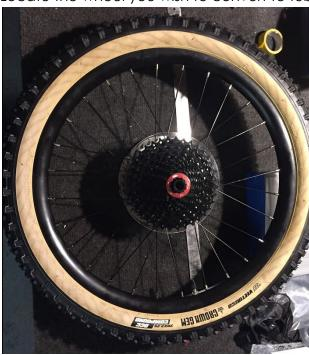
2. Unscrew the presta valve head, and remove all the air from the tyre by pressing the valve core.
