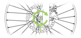
Slide the 15mm axle into the fork from the left hand side (disc side), gently turn the axle to engage the first few threads, then tighten to 12-15Nm. Once tight, check the disc brake operates correctly.
