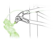
2 Using the 5mm allen key, Fit the derailleur into the mech hanger but do not tighten yet.
