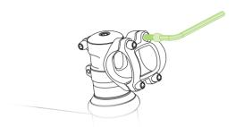
Remove protection from stem and remove the protective wrapping from the handlebar. Remove the stem bolts using the 4mm allen key and put them somewhere safe.
