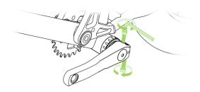
Using the supplied 5mm allen key. Remove the 2 pinch bolts.
