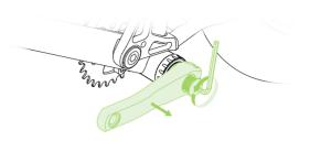
Remove the crank preload bolt. Then remove the non drive-side crank arm.
