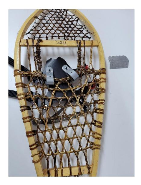
3- Fold the grey straps in half, so you can pass the screws trough the harness and the straps
