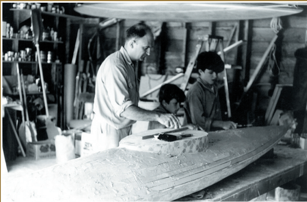
In the garage, Werner Sr. with Bruce and Erich building the plug for the form of the first fiberglass kayak in 1966.
