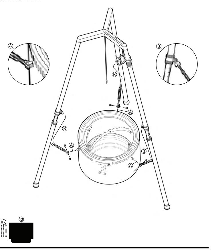
${\sf A}$  Connect the turnbuckles to the sides of the barrel.
