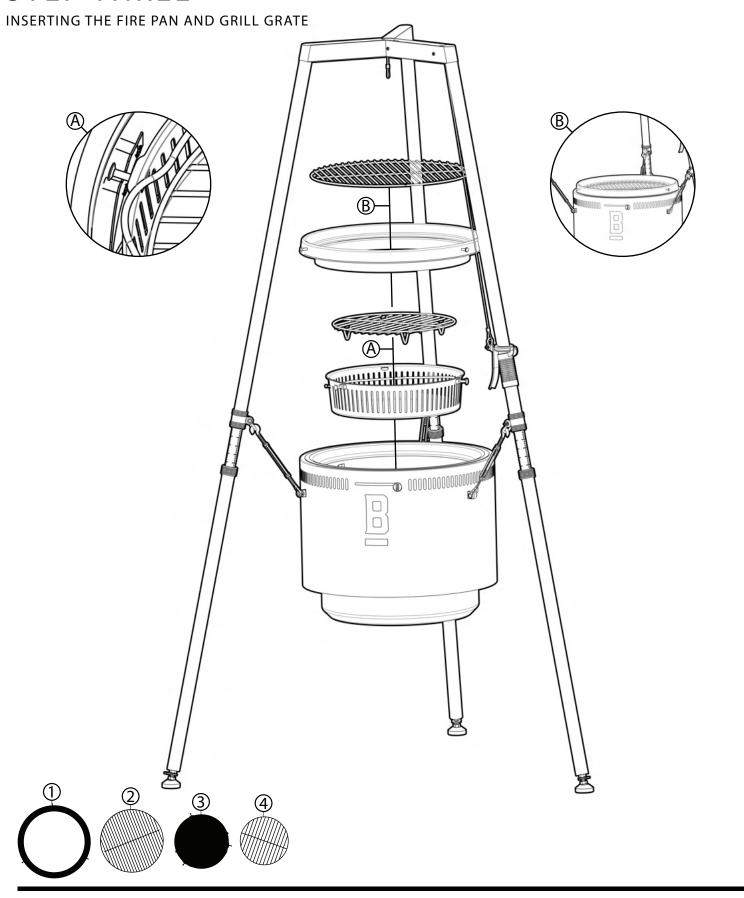
A Place the fire pan and fire pan grate together on the spiral tracks. Spin the fire pan to adjust the height.
