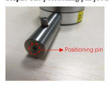
**Step3:** Insert the ferrule into bottom of measuring rod and push the positioning pin up, then screw the fixed button to keep positioning pin still.
