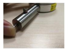
**Step4:** After finishing the steps above, we can start to measure the ferrule length. Insert the ferule into bottom of measuring rod, then read the test value on screen.
