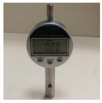
Step2: The positioning pin protrudes the bottom of measuring rod at the initial state.
