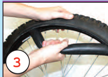
3. Slowly remove the inner tube
