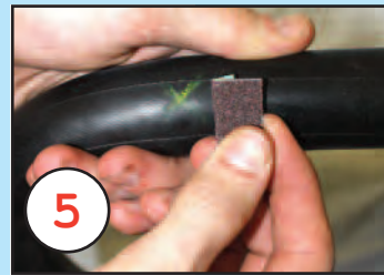
5. Roughen the surface around it with sandpaper
