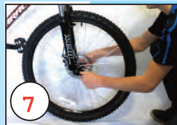
7. Put the tyre back on the rim and back on to the bicycle
