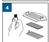
Use the cleaning tool to brush the filter cover and filters. Do not wash the filters.
