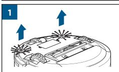
Use a Phillips-head screwdriver to remove the screw. Pull up on the base of the brush.
