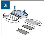
Remove the filter cover, then the foam and pleated filters.
