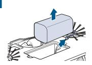
Remove the battery and disconnect.
