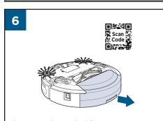
The QR code needed for setup can be found by removing the dirt bin and turning the robot over.
