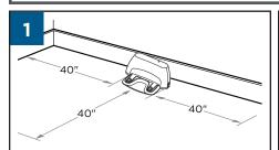
Place the back of docking station firmly against a wall. Ensure there are at least 40 inches to one side, 40 inches to the opposing side and no obstructions in front of the docking station.
