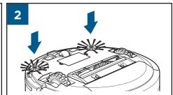
Push the brush directly onto the holder. Replace the screws with a Phillips-head screwdriver.
