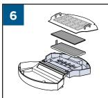
Once clean, reinstall the filters and filter cover. close and push back into the machine.
