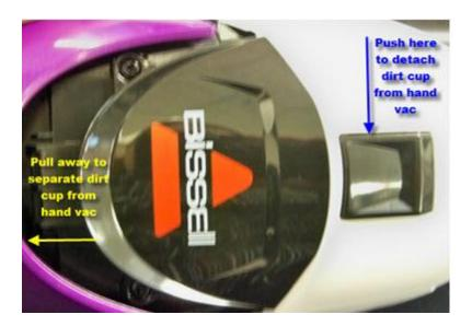
Make sure the dirt cup is properly attached to the hand vac. It should click properly into place and the dirt cup should have no space between where the dirt cup meets the battery pack. (See picture below).
