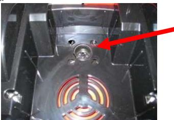
E) Is there SUCTION at the MOTOR DUCT GASKET?
