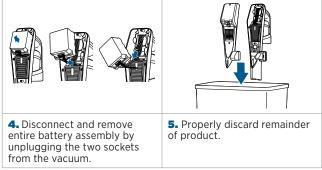
NOTE: Keep Battery Pack together – DO NOT separate individual batteries.
