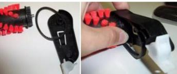
7. Next, position the brush roll so that the belt side is on the same side as the pulley and slowly lower the brush down into place. Once lowered the belt can be attached to the brush roll and the clips can be slid into place and screwed in. Replace the red clip in it's proper location and screw it down too.
