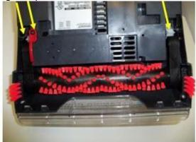
3. Slide the brush roll and pivot arms holding the brush roll in place out of the unit remove the old or broken belt. The belt attached directly to the brush roll should have grooved teeth and connect to the pulley that sat where the larger red clip was pulled out from.
