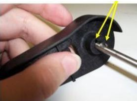
9. **Rotate the brush roll towards the motor pulley** to align the belts and ensure the brush roll rotates freely.
