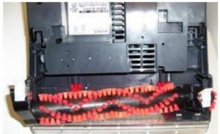
4. Once the brush and brush belt is removed, the pump belt can then be removed. This can easily be done by sliding it off of the pulley on the top side of the unit in the belt access door first. Then with the unit turned over slide it off the pulley where the brush belt attaches.
