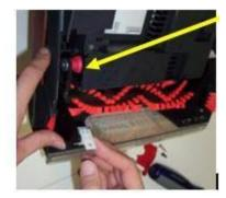
8. **Lift the brush roll upwards after all screws are attached** to see if the brush roll can move up and down freely without rubbing on the sides of the unit. If the sides rub the metal rod inside the brush roll is not inserted properly into its groove causing it to push the end caps outward and will cause the rubbing.
